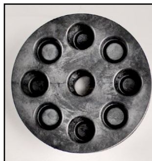
RETAINER AND COVER INTERLOCKED
