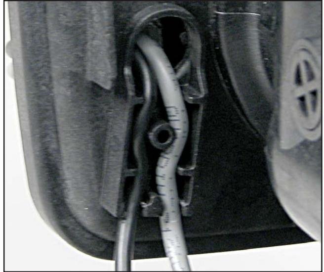
9a. Breakout second tab of "ALT b" strain relief on the backside of the backplate to allow the water meter cable to be weaved through.
