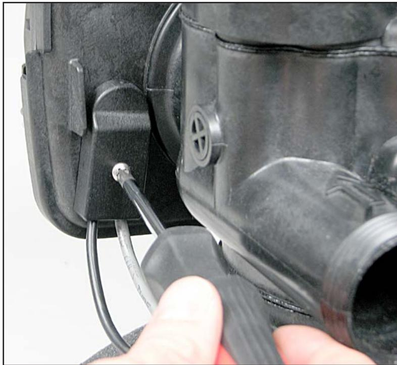
9b. Then fasten the strain relief cover over the top of the strain relief.
