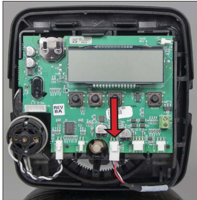
7. For control valve "ALT b" the other end of the interconnect cable needs to be routed through the knockout hole on the backside of the backplate. Connect the end of the interconnect cable to the three pin connection labeled "INTERCONNECT CABLE" on the PC Board.
