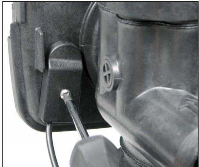
8. On the backside of "ALT b" you will need to breakout only one tab at the bottom of the strain relief for 1" and 1.25" control valves. This will allow to weave the interconnect cable down through the strain relief so you can install and fasten the strain relief cover over the top of the strain relief. See step 9 (pg. 9) for 1.5" and 2" control valves.
