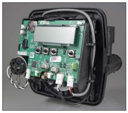
5. Re-install the drive bracket assemblies and re-connect any disconnected wires back to the proper location on each PC Board.
