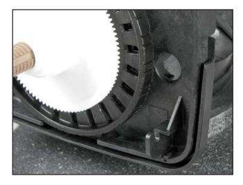
3. Once drive bracket is removed, locate knockout on backplate. You can use a punch or a Phillips screw driver and place it in the center of the knockout circle and tap it with a mild to medium force with a hammer to punch out circle knockout piece.
