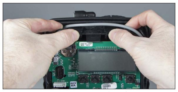
2. You will need to remove the valves drive bracket and PC Board from the backplate and disconnect the wires from the PC Boards.
