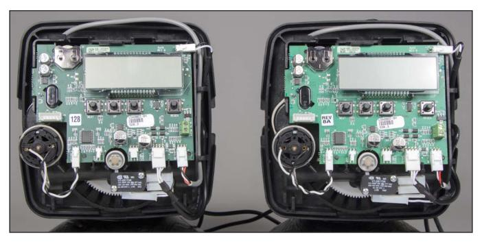
10. The wire shield that was not shown needs to have the wires installed into it in the proper positions and then installed on each valve's micro switch. Next the wire with the white Molex connector end needs to be connected to each PC Boards two pin connector for the DP switch. Make sure all wires are connected to the proper connections before powering the valves and beginning to program.
