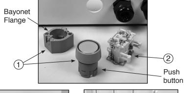
Ensure Push button \_\_\_\_ is flush to enclosure
